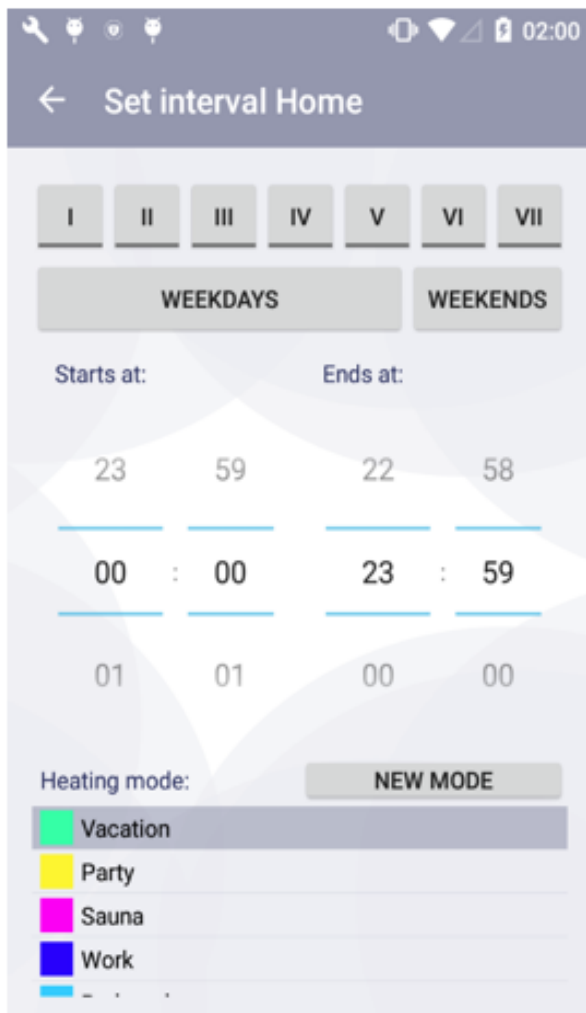
Figure 19. The window for creating a heating period used in the weekly heating program
