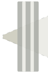
Reinforced concrete loss: 40 to 90%
