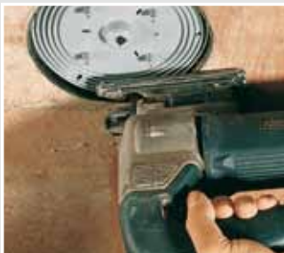
Open front part using a fretsaw.
