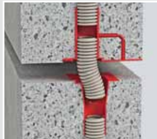
Compensation in transverse direction \pm 10 mm.
