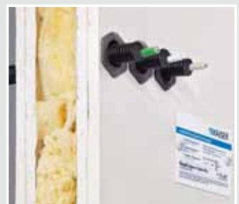
Three conduit sealings can be arranged vertically or horizontally to form a group with a centre distance of 50 mm.
