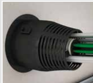
Fit the two-part sealing element round the bundle, close it and connect it to the sealing cylinder by means of the bayonet fitting.
