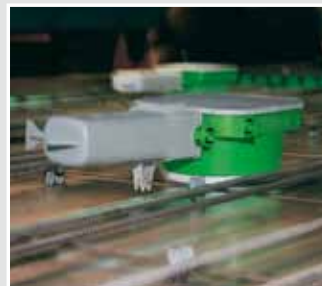
Clip the tunnel support onto the distance rod using the enclosed spacer.
