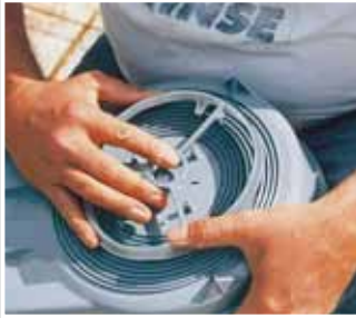
Clip the front ring onto the housing.
