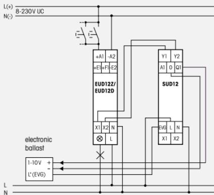
In this mode electronic ballast and transformers with a 1-10V interface up to a total control current of 40mA can be controlled when connected to an universal dimmer switch EUD12Z or EUD12D.
