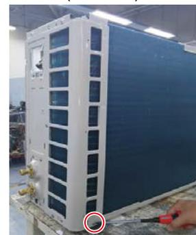
4) Disassemble the screw fixing ring, then take the ring out as below picture direction.
