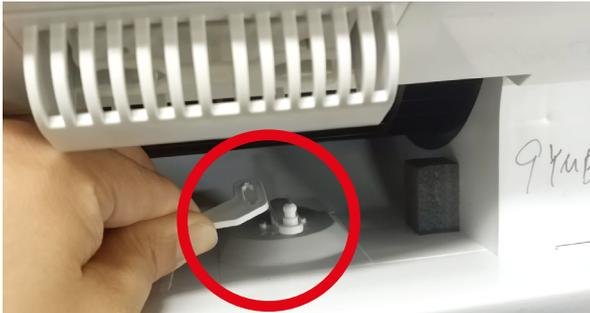
23) Hold and press the Cross Flow Fan to left side as much as possible, meanwhile, take Fan Motor out.
