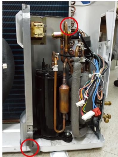
12) Remove the screw fixing Motor Angle, then take it out.
