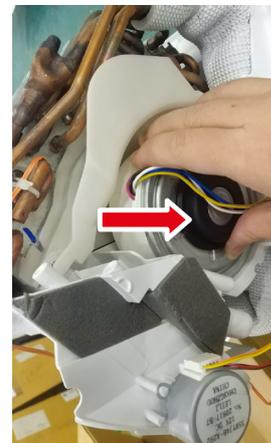
20) Remove the 2 screws of Louver Motor V to take the motor out.
