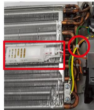
9) Remove 2 screw fixing the Ground wire.
