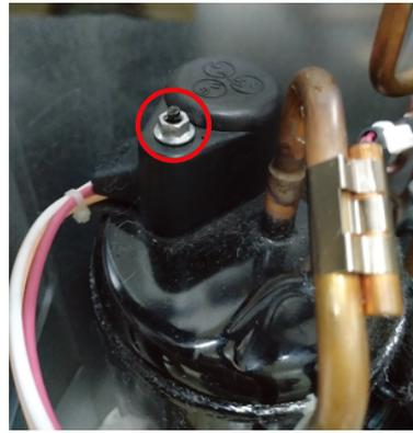
10) Disconnect three terminals on the Compressor.
