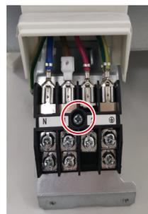
4) Disassemble terminal holder, if terminal holder broken.(1 screw)
