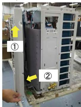
3) Disassemble the top cover after removing 4 screws of it.
