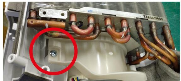
21) Remove 2 screw fixing the Fan Motor Cover, then remove Fan Motor Cover.
