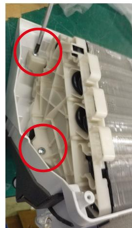
22) Remove 1 screw between Cross Flow Fan and Fan Motor.
