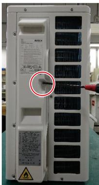
5) Disassemble the front cabinet ass'y.(5 screws in front side, 4 screws in right side.)
