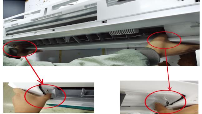
8) Cut the Wire Fixing Band and remove the Thermistor.
