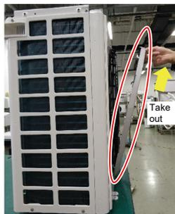
7) Disassemble side cover L.(6 screws)
